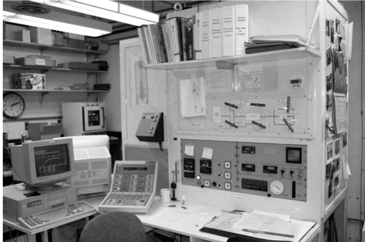
*Gas medium High pressure Torsion apparatus (UMN)*
